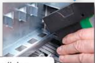
Install the conversion modules into the baseplate.
