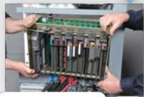
Remove the 1771 chassis from the control cabinet.
